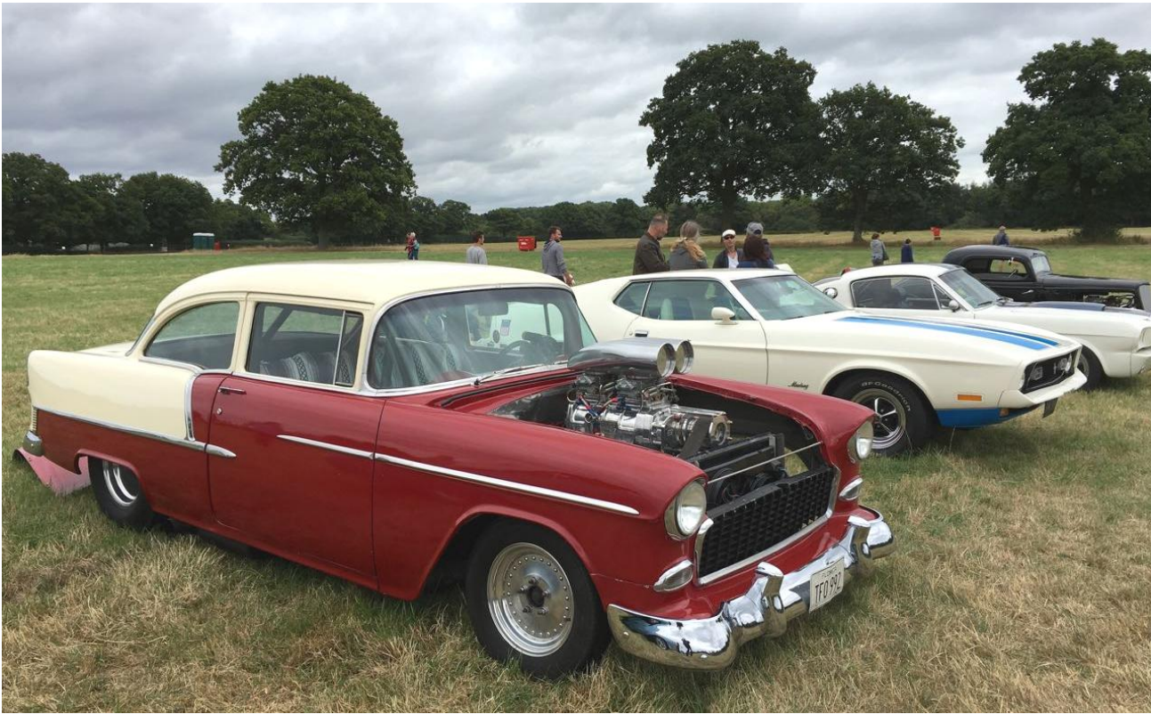
Rod Currie's '55 Chevrolet 210 street machine packs a 540-cube 850-plus horsepower Chevy big block put together by master engine builders Jeff Bull and Tony Gransden Roger Phillips photo
