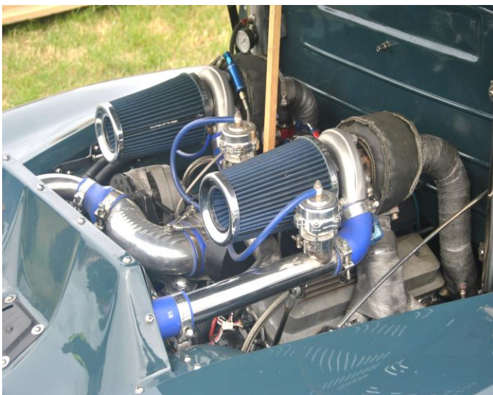
Mark Steven’s shot (above right) shows Adrian Wright’s 480bhp LS376 Chevy crate motor neatly shoe-horned into his 1967 Vauxhall Cresta PC Estate along with a six-speed Tremec gearbox
