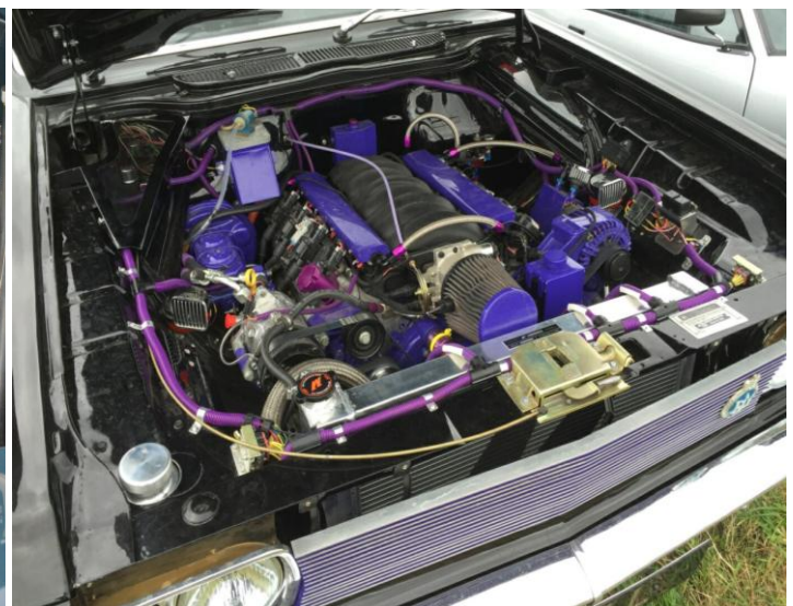
Mark Steven’s shot (above right) shows Adrian Wright’s 480bhp LS376 Chevy crate motor neatly shoe-horned into his 1967 Vauxhall Cresta PC Estate along with a six-speed Tremec gearbox
