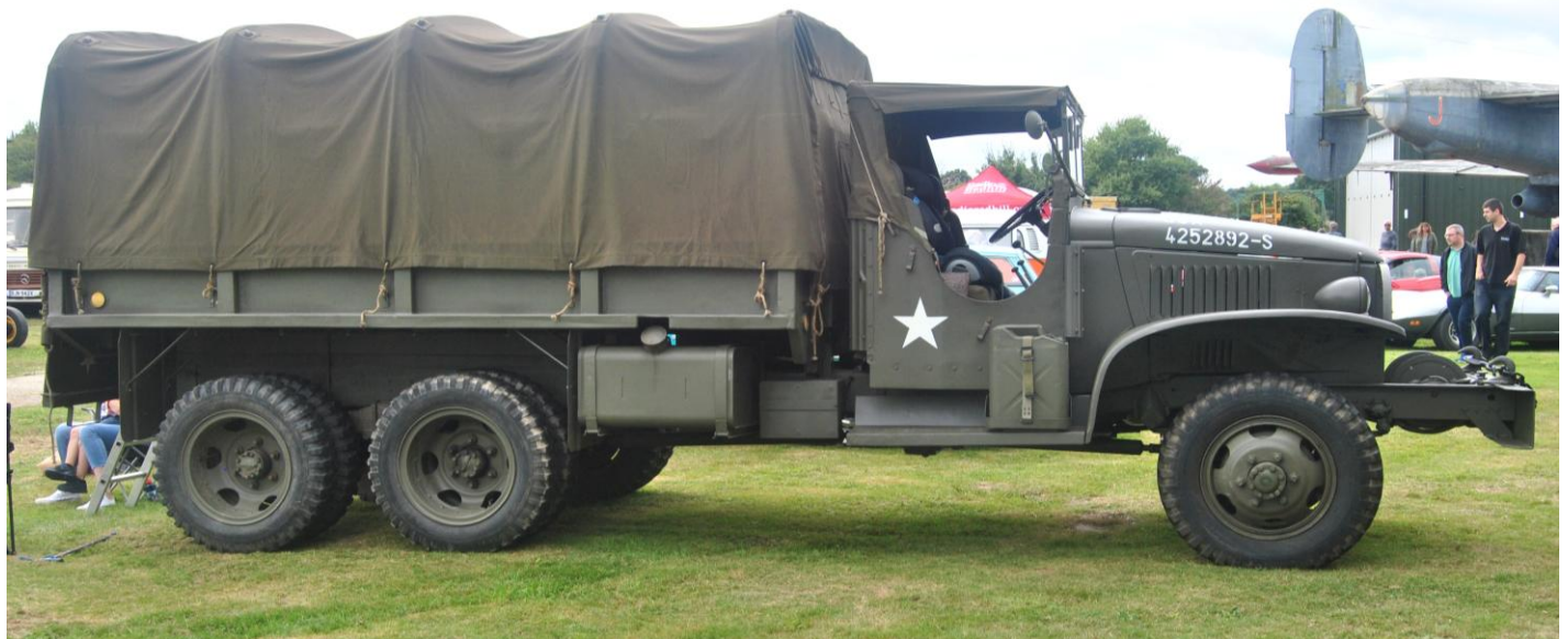
On the subject of Deuces, this is an ex-US Army World War II pattern "Duece-and-half", so named because it has a two-and-a-half ton payload, and this is one of more than half-a-million produced in virtually-identical form by GMC, Chevrolet and Studebaker. The "4 th US Infantry" re-enactors, with Jeeps and Dodge Weapons Carriers, created a realistic battlefield checkpoint within the showground woodlands in an encampment coordinated by Kevin Rowlett. Thanks Kevin Wojtek Samoszuk photo
